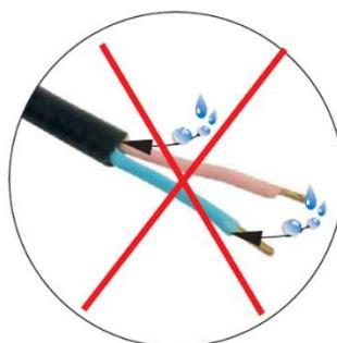
Be sure to use an IP68 cable connector. Temperature changes in the stone can cause moisture to be drawn in through the insulation, which can damage the luminaire.
